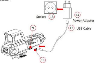
**Note:** 1. When the USB-C cable is used for power supply, the scope switches the power supply from the battery to the USB-C cable.
